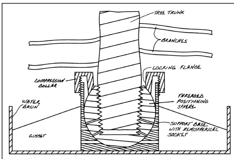
is joining a sphere to the end of the tree trunk, placing the sphere in a matching socket, and providing a reversible means for locking the sphere in position in the socket, releasing it for adjustment, and re-locking it.
